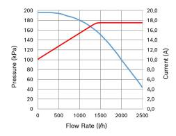
Flow rate (I/h): 1200 Nominal pressure (bar): 1.7 Nominal Voltage (V): 12 Weight (kg): 0.7 Control: PWM Medium: Water/Glycol (50/50)
