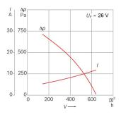
Nominal Voltage (V): 24 Nominal current (A): 8 Nominal speed (rpm): 4468 Air flow (m3/h): 400 Pressure difference (Pa): 470 Hall Sensor: No
