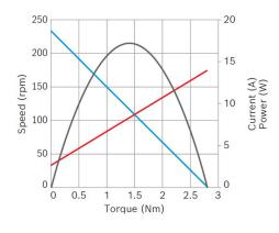
Nominal power (W): 6,6 Nominal current (A): 3,8 Nominal speed (rpm): 210 Nominal torque (Nm): 0,3 Stall torque (Nm): 2,8 Transmission ratio: 28:2 Hall Sensor: Yes Transmission position: Left
