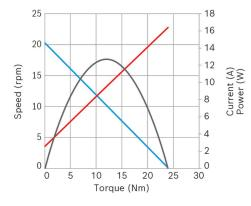
Nominal power (W): 3,9 Nominal current (A): 3,7 Nominal speed (rpm): 18,65 Nominal torque (Nm): 2 Stall torque (Nm): 21,5 Transmission ratio: 217:1 Hall Sensor: Yes Transmission position: Right
