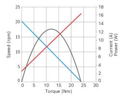
Nominal power (W): 3,9 Nominal current (A): 3,7 Nominal speed (rpm): 18,65 Nominal torque (Nm): 2 Stall torque (Nm): 21,5 Transmission ratio: 217:1 Hall Sensor: Yes Transmission position: Left
