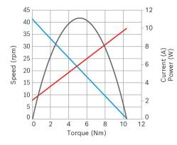
Nominal power (W): 3,9 Nominal current (A): 2,8 Nominal speed (rpm): 37,3 Nominal torque (Nm): 1 Stall torque (Nm): 10,35 Transmission ratio: 182:2 Hall Sensor: No Transmission position: Right
