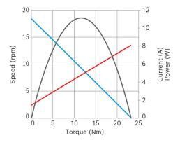
Nominal power (W): 3,5 Nominal current (A): 2 Nominal speed (rpm): 16,9 Nominal torque (Nm): 2 Stall torque (Nm): 23,3 Transmission ratio: 217:1 Hall Sensor: Yes Transmission position: Right
