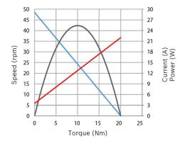
Nominal power (W): 9,1 Nominal current (A): 5,4 Nominal speed (rpm): 43,8 Nominal torque (Nm): 2 Stall torque (Nm): 20 Transmission ratio: 91:1 Hall Sensor: Yes Transmission position: Right
