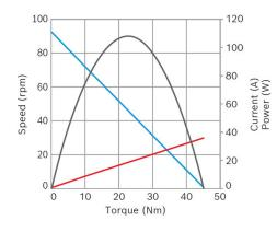
Nominal power (W): 38,7 Nominal current (A): 8,5 Nominal speed (rpm): 37 Nominal torque (Nm): 10 Stall torque (Nm): 40 Transmission ratio: 78:1 Hall Sensor: 2x Rotation direction: Left and right rotation
