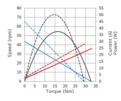
Nominal power (W)\*: 12,8 / 8,5 Nominal current (A)\*: 4,5 / 3,5 Nominal speed (rpm)\*: 61 / 41 Nominal torque (Nm): 2 Stall torque (Nm)\*: 25 / 28 Transmission ratio: 76:1 Rotation direction: counterclockwise Hall Sensor: No Transmission position: Left \*Motor with two speeds
