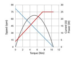
Nominal power (W): 8,6 Nominal current (A): 6 Nominal speed (rpm): 82 Nominal torque (Nm): 1 Stall torque (Nm): 10 Transmission ratio: 73:1 Transmission position: Right
