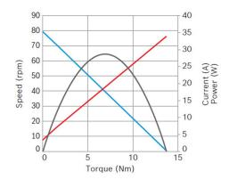
Nominal power (W): 7,8 Nominal current (A): 6 Nominal speed (rpm): 74,5 Nominal torque (Nm): 1 Stall torque (Nm): 13,7 Transmission ratio: 73:1 Hall Sensor: No Transmission position: Left
