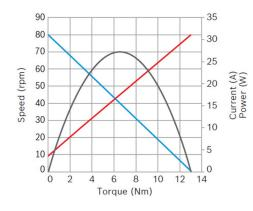
Nominal power (W): 7,8 Nominal current (A): 6 Nominal speed (rpm): 74,5 Nominal torque (Nm): 1 Stall torque (Nm): 13 Transmission ratio: 73:1 Hall Sensor: 2x Transmission position: Right
