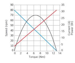
Nominal power (W): 7,8 Nominal current (A): 6 Nominal speed (rpm): 74,5 Nominal torque (Nm): 1 Stall torque (Nm): 13 Transmission ratio: 73:1 Hall Sensor: 2x Transmission position: Left
