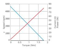
Nominal power (W): 122,5 Nominal current (A): 115 Nominal speed (rpm): 3900 Nominal torque (Nm): 0,3 Stall torque (Nm): 1,8 Hall Sensor: No
