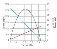
Nominal power (W): 12,6 Nominal current (A): 2,5 Nominal speed (rpm): 2400 Nominal torque (Nm): 0,05 Stall torque (Nm): 0,43 Hall Sensor: Yes
