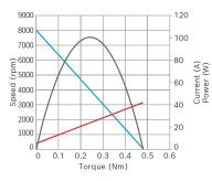
Nominal power (W): 37,7 Nominal current (A): 9 Nominal speed (rpm): 7200 Nominal torque (Nm): 0,05 Stall torque (Nm): 0,43 Hall Sensor: Yes
