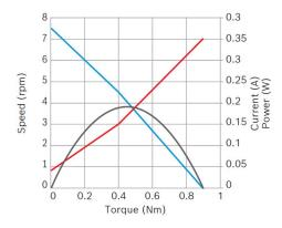
Nominal power (W): 0,2 Nominal current (A): 0,15 Nominal speed (rpm): 4,5 Nominal torque (Nm): 0,4 Stall torque (Nm): 0,9 Transmission ratio: 405:1 Degree of protection: IP 40 Signal potentiometer: Yes
